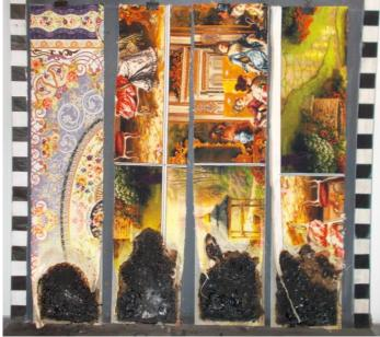
2.3 Reaction to fire tests – Ignitability of building products subjected to direct **impingement of** flame
